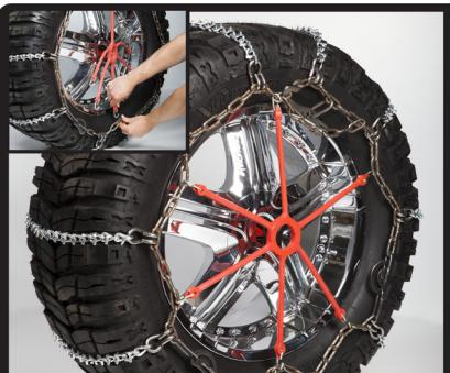
**7** Repeat step 6 on the front side of the tire. Use tie strap to secure left over side chain.
