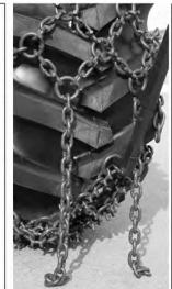
Use a tensioning device (not included) to bring the rings close together. This will tighten up the main pattern.
