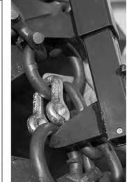
10A If you can, couple the chain together ring to ring with either a shackle or plug coupler provided.
