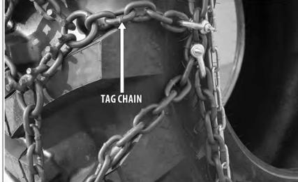
12 Last step is to cut your side chain  $\angle$ or tie it back so it doesn't flail. Also, if you connected your main pattern ring to ring, cut the tails completely off.
